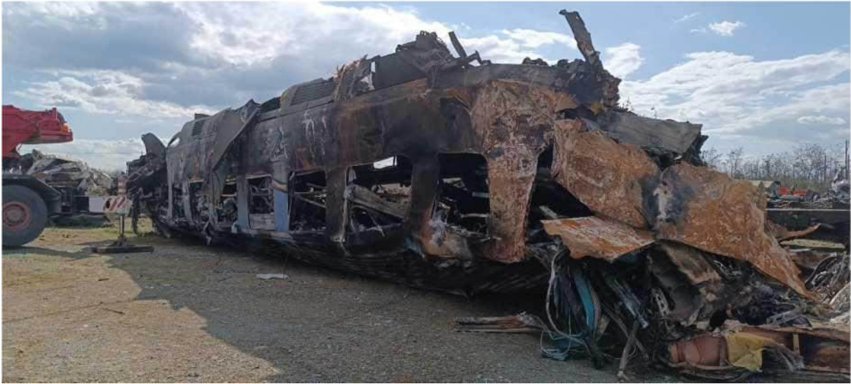
Figure 87. Position 4) B2 2nd class coach, heavy impact damage in the front and rear, fire slowly consumed it.
