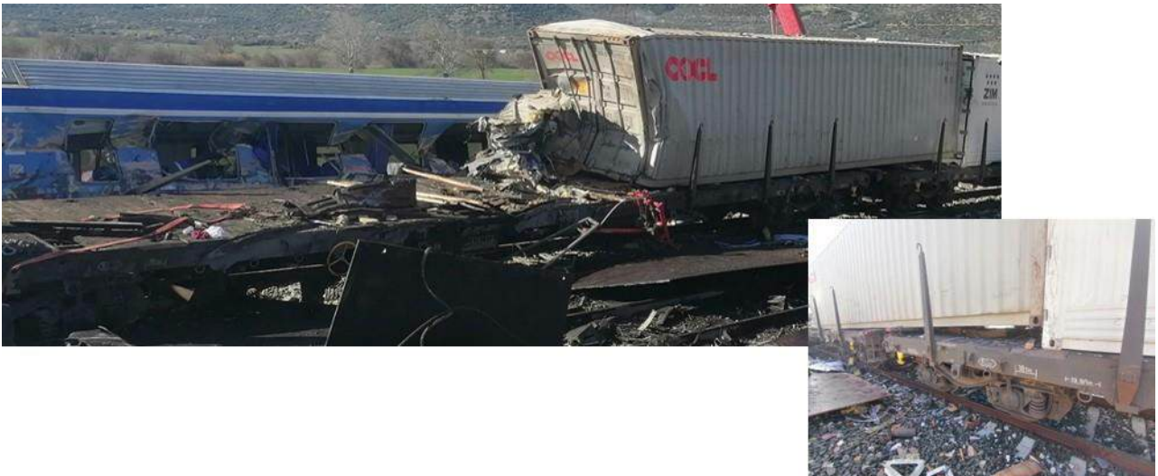
Figure 83. Positions 6) and 7) – on the left, the platform nr 4 (damaged, lost front bogie, not derailed) carrying the first container. On the right, the first container (OOCL) is shifted in rear direction, hurting the next container (ZIMonitor).
