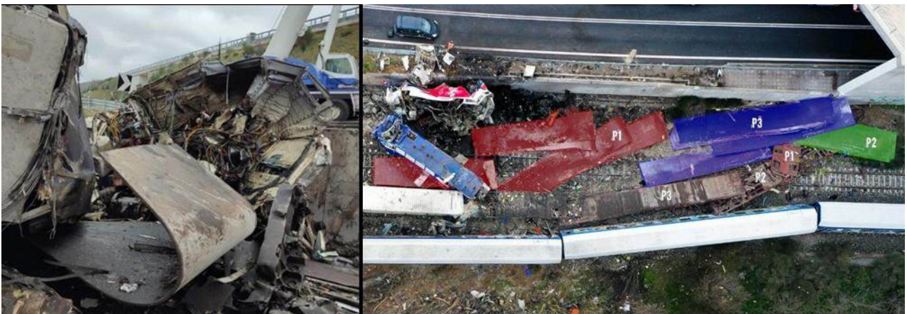
Figure 22. Remains of the top steel plates and final position of the 3 sets of steel plates.
