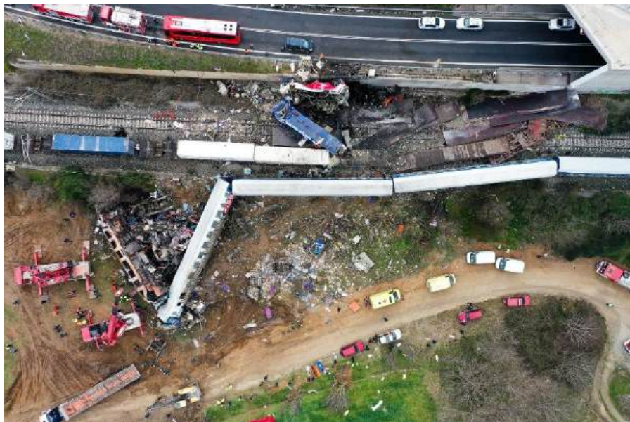
Figure 10. The end position of the 3 locomotives and some of the passengers coaches and freight wagons ( http://www.intime.gr/ ).
