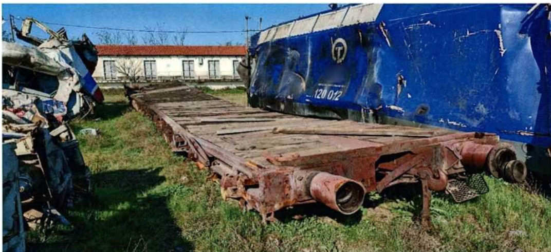
Figure 81. Position 5) nr 3 platform carrying steel plates, lost bogies from derailment, slight damage (twist) due to crash from the rear.
