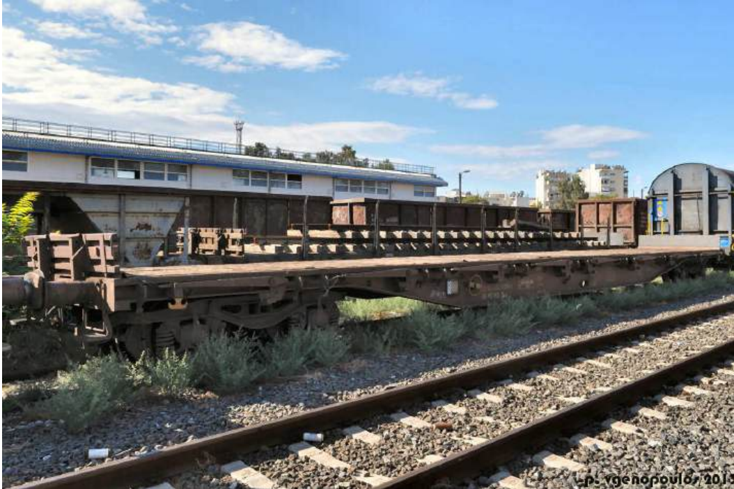
Figure 71. Type of platform supporting the steel plates (For the steel plates: WAGON 31 65 xxx MZ , https://hellas-express.eu/viewtopic.php?f=15&t=43&p=1162&hilit=454#p1162 ).
