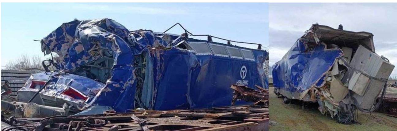
Figure 78. Position 2) 120 012 locomotive, heavy damage in the front (with locomotive 120-022) and rear, signs of crash against 1st container on P4, without the missing rear cab.
